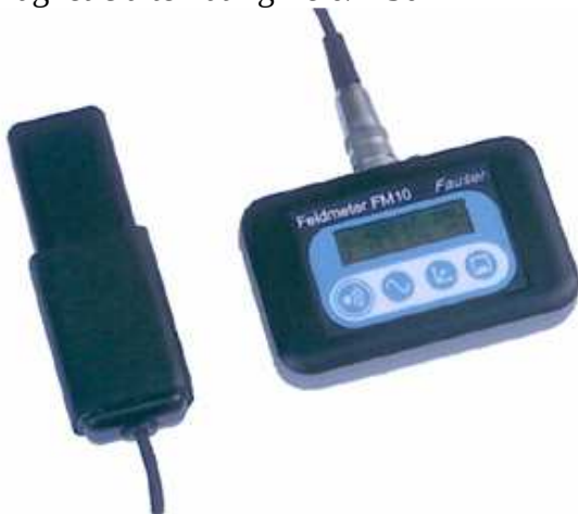
Модель Feldmeter FM 10L Fausel. www.rayonex.co.uk -Isotropic magnetic field measurement Potential related and floating electric fields -Frequency range from 10 Hz to 400 kHz Resolution from 1 nT and 0.1 V/m, resp. without measuring range change -Data logger for continuous recording and single point measurement with huge 1 GByte memory capacity -Filters for 16.6 Hz, 50 Hz and 2 KHz
